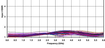
Figure 5. Input VSWR vs. Frequency Over All Attenuator States
